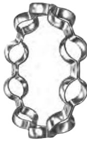
Fig. A-2. Pressed-steel welded cage.
